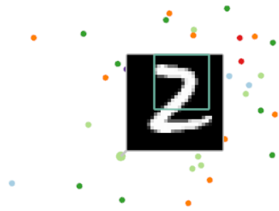
Fig. 3. The receptive field associated with a representation of an MNIST digit. Note that features firing for this particular receptive field could equally point towards identification as a two or a seven, and that further context will need to be incorporated in further layers to disambiguate the digit.
